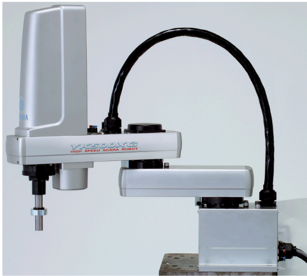
Figure 3.15: The Yamaha© YK500XG is a high-speed SCARA robot with two revolute joints and a vertical prismatic joint. Image courtesy of Yamaha Motor Co., Ltd, http://
