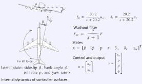
In this example, there is no sensor to measure  $x_w$ . Also, the sensor that we have measures  $r_w$  rather than r.
