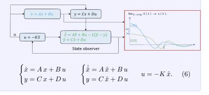
To study whether the system (6) with output feedback  $u = -K \hat{x}$  is exponentially stable, form the close-loop system matrix with states x and  $e = \hat{x} - x$ :
