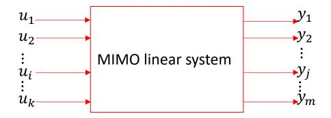
**Impulse response for MIMO** : mathematical description of zero-state response for a system with k input and m output (**linear**, **causal** and **relaxed** system)
