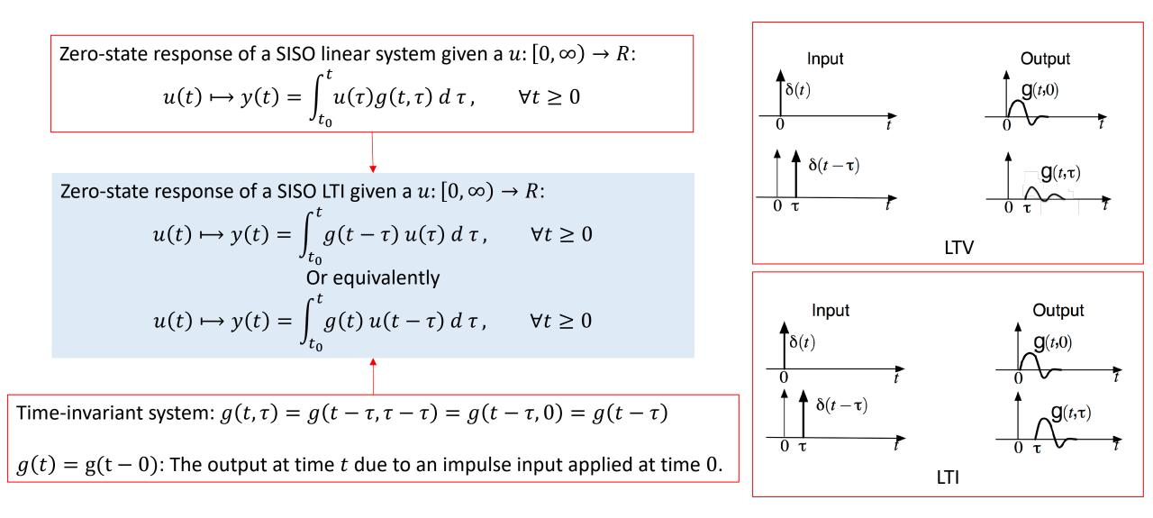
Input-output description (Impulse response) for relaxed and linear system
